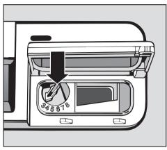
The dosage adjuster (see arrow) in the opening has settings adjustable from 1 to 6 (1-6 ml). It is set to "3" (3 ml) at the factory as the recommended dose.
